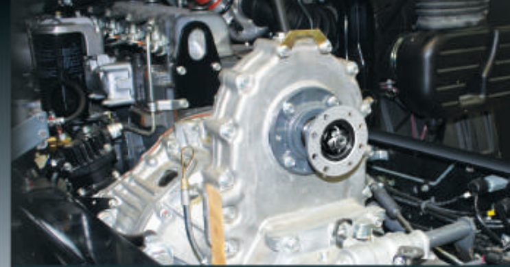
Full Power PTO (FM 657H only) This full power PTO has an output speed ratio of 1:1.195 (Engine Speed : PTO Speed) Ideal for firetruck, sludge extraction, or concrete pumping application.
