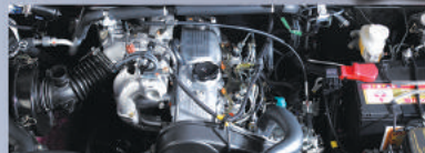
Powerful yet Economical 4D54 which is now Euro-2 Compliant 2.5-Liter 4-In-Line Diesel Engine, Distributor Type Fuel Injection
